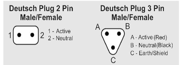
Cables are colour coded for easy identification. When installing system, cables should be only connected to the correctly coded cable. Colour Coding for cables is as follows:
