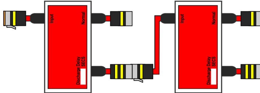
The FP-0450/8451 fire control panel activation sequence is limited to prevent accidental discharges when servicing. The maximum amount of time power is supplied to the activation circuit is 4.5 minutes. **Any programming to the Discharge Delay modules must not exceed this time limitation, or the modules will not operate.** (For example; if programmed M1 – 2.5min, M2 – 2.5min, M3 – 2.5min; module 3 will not operate).
