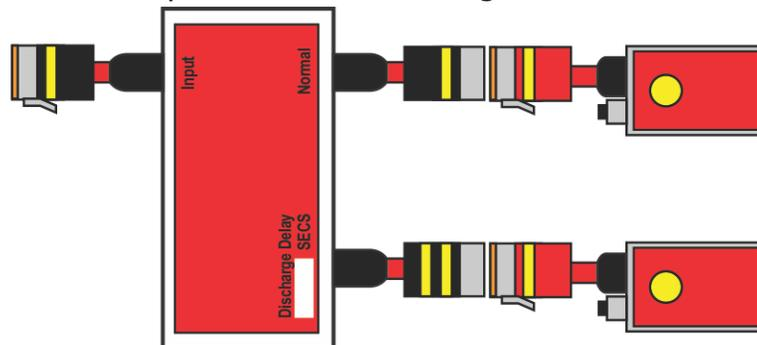
4. If only using the "Delayed Discharge" output, the  $3k3\Omega$  End-of-line resistor should be terminated into the supplied 3 pin deutsch plug and then connected to the "Normal" output on the module (marked yellow 1). The end-of-line plug should then be covered in heatshrink, and the heatshrink crimped, to avoid ingress of water into the circuit.
