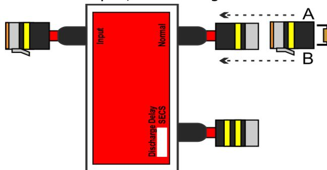
5. If using multiple modules, the next module should now be connected to the "Discharge Delay" output on the first module and step 2 repeated.
